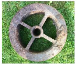
The wheel, photographed here, is now with 'The Friends'. We have no reason to doubt the authenticity of where and when it was found, but it has thrown up more questions. Constructed out of cast iron with a replaceable steel 'tyre' bolted in place, it weighs about 120 lbs., and has four spokes, but with a diameter of only 19 inches it does seem on the small side for use on a horse drawn tramway wagon.
