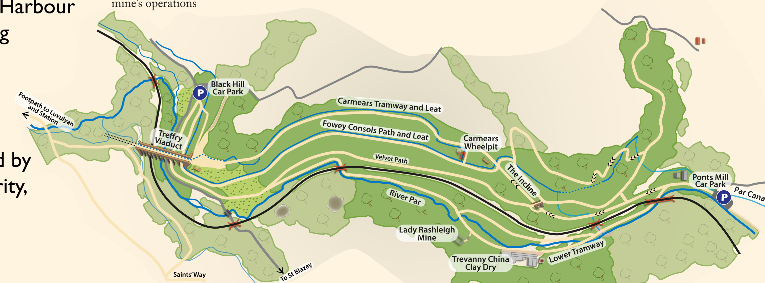
Aerial view of Treffry Viaduct, built 1839-1842, to enable rail access to the china clay and stone reserves in the Hensbarrow district and to link with Treffry's harbour at Newquay. The Viaduct also carried water to power the Carmears Inclined Plane, after which it flowed into the Fowey Consols Mine leat to provide additional water essential for the mine's operations
